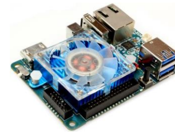
ODROID-XU4 Single Board Computer with Quad Core 2GHz A15, 2GB RAM
